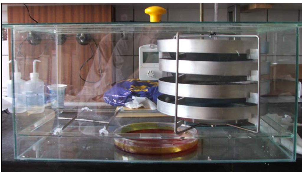
FIG. 3: Final experimental apparatus for water vapour permeability measurement with only one tray of cups.
