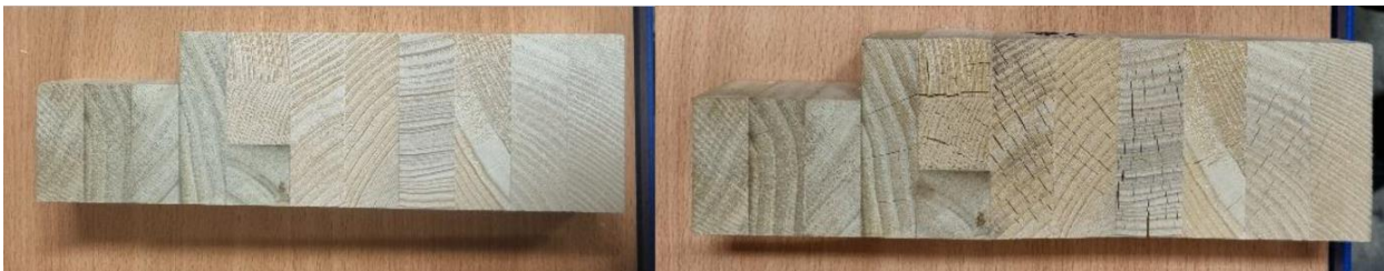
Fig.16. One sample of glulam timber before (left) and after (right) the boiling test. The other three samples looked very similar.
